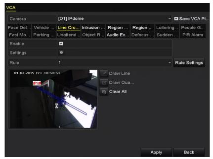
Figure 9-7 Draw Line for Line Crossing Detection
