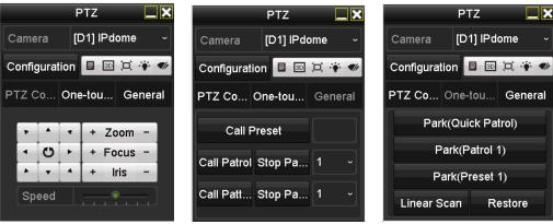
Figure 4-14 PTZ Control Panel
