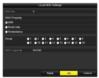
Figure 12-13 Local HDD Settings Interface
