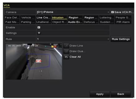
Figure 9-9 Draw Area for Intrusion Detection
