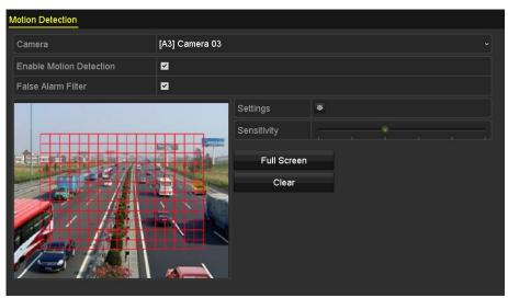
Figure 8-2 Set Detection Area and Sensitivity
