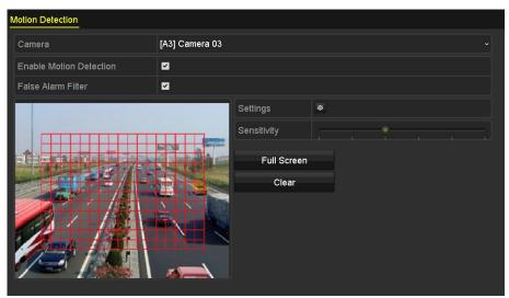
Figure 5-14 Motion Detection- Mask
