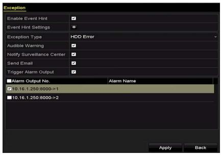
Figure 12-26 Configure HDD Error Alarm
