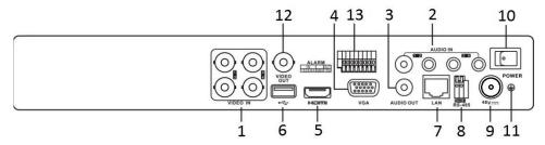
Figure 1-5 Rear Panel of HDDVR4
