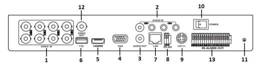
Figure 1-6 Rear Panel of HDDVR8
