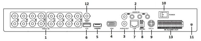
Figure 1-7 Rear Panel of HDDVR16
