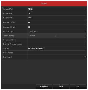
Figure 2-23 Set Advanced Network Parameters
