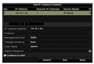
Figure 2-41 Custom Adding IP Camera Interface
