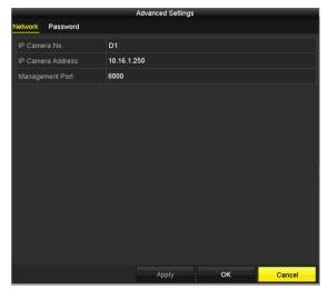
Figure 2-44 Network Configuration of the Camera
