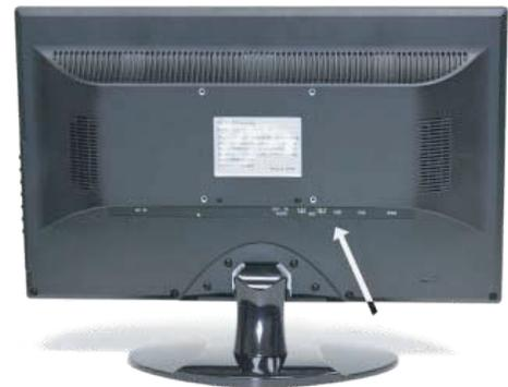
Use **ONLY** a properly grounded three wire cord appropriate for the local power system.
