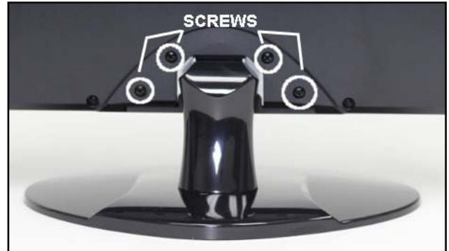
2. Attach the VESA mount (100mm x 100mm) plate to the rear of the monitor and follow all of the instructions provided with the mount to complete the mounting process.
