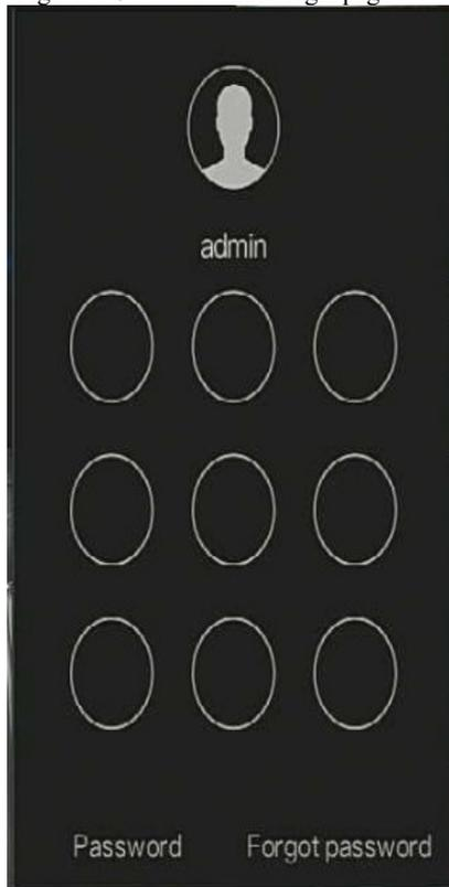
Step 2 On the DVR login page, click “ Password” to at pattern unlock interface. If user don’t set the pattern unlock it will show password to login interface directly, select the language, as shown in Figure 4-7.
