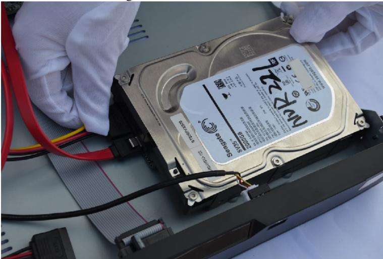
Step 5 Insert the hard disk data cable and power cable, then put on the upper cover and fasten the fixing screws.
