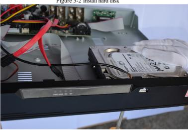
Figure 3-2 Install hard disk
