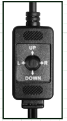
In-Line Cable Mounted OSD Control
