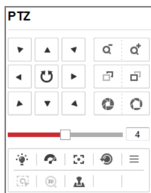
Figure 5-3 PTZ Control Panel
