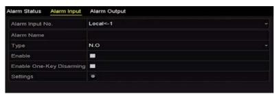
Figure 8-5 Alarm Input Setup Interface
