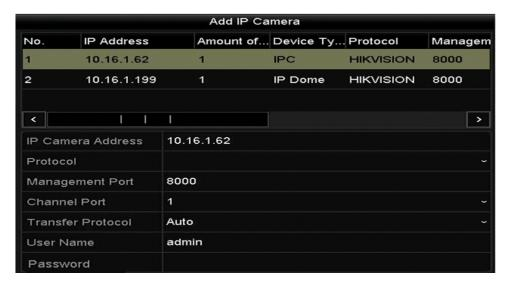
Figure 2-26 Quick Adding IP Camera Interface
