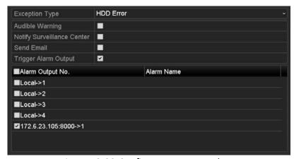
Figure 12-29 Configure HDD Error Alarm
