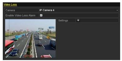
Figure 8-9 Video Loss Setup Interface
