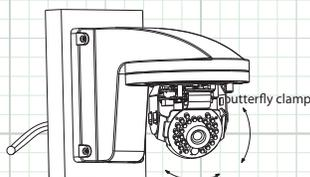
5. Install the housing and lock the screws.
