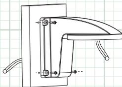
2. Loosen the tightening screw and take down the housing.
