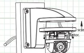
4. Adjust the angle through the 3-axis adjustment structure.
