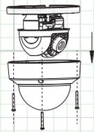
3. Install the dome core to the gang box, wire and lock the screw.
