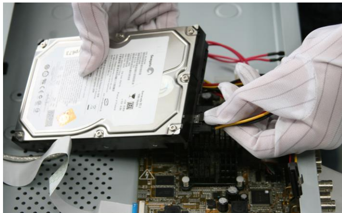
Figure 2. 3 Connect Power Cable
