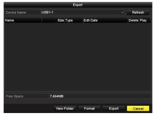
Figure 7. 15 Export Video Clips Using USB Flash Drive
