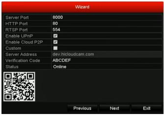
Figure 2. 8 Advanced Network Configuration
