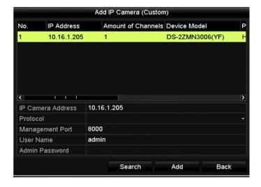
Figure 2. 19 Custom Adding IP Camera Interface
