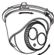
Figure 2. 17 Adjust the viewing angle
