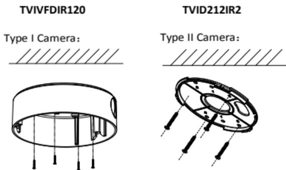
Figure 2. 2 Attach the Back Box/Base Plate
