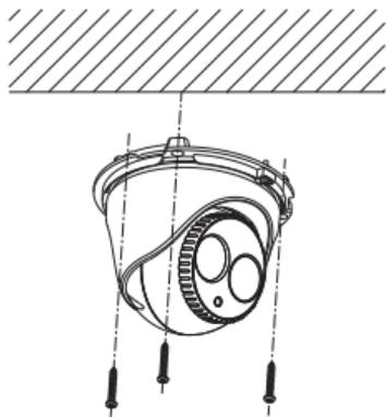
Figure 2. 15 Secure the camera to the Ceiling
