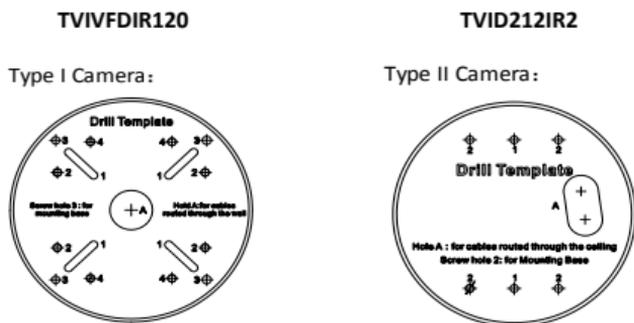
Figure 2. 1 The Drill Template
