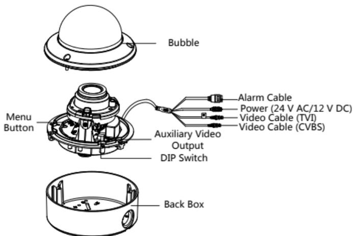
Figure 1. 1 Overview of TVIVFDIR120 Outdoor Dome Camera
