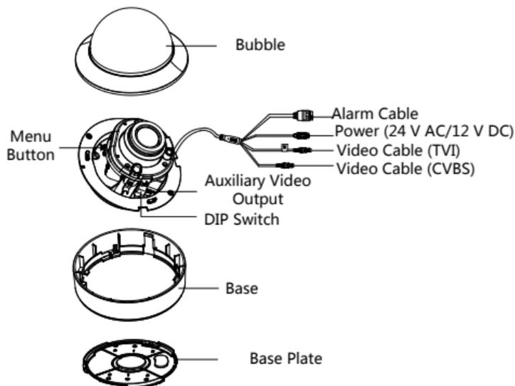
Figure 1. 2 Overview of TVID212IR2 Indoor Dome Camera
