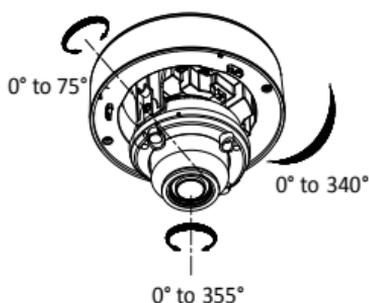
Figure 2. 4 3-Axis Adjustment
