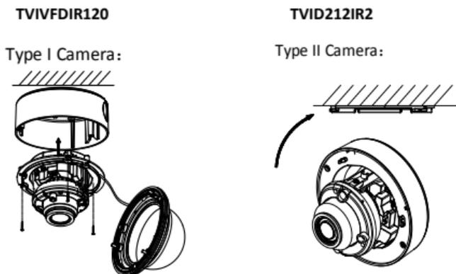
Figure 2. 3 Fix the camera to the Ceiling
