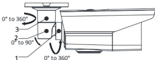
Figure 2. 10 3-Axis Adjustment
