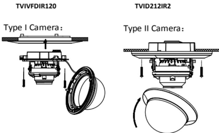
Figure 2. 6 Fix the Camera to the Mount
