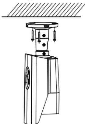
Figure 2. 8 Fix the Camera to the Ceiling
