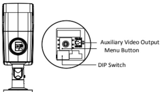
Figure 2. 9 Internal Interface and Button
