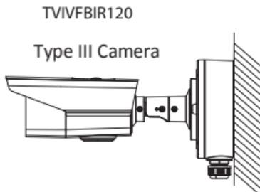
Figure 2. 12 Wall/Ceiling Mounting with the Junction Box
